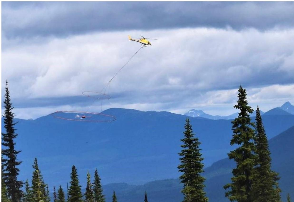
*An AStar B3 helicopter completing the VTEM and Magnetic Geophysical Survey at the Stardust Project – July 2018*
